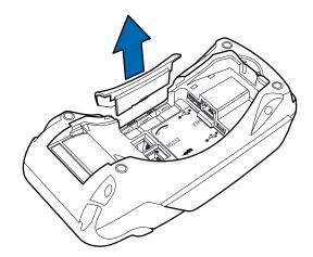
Figure 13 Removing MSAM Cover
