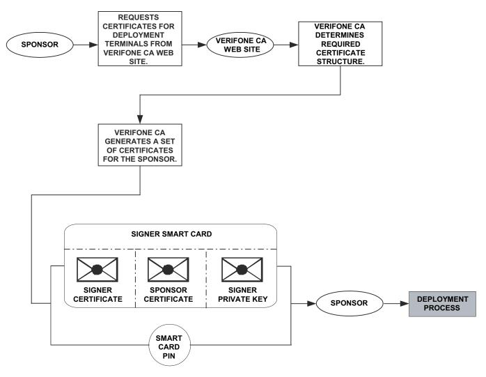
Figure 28 The Pre-Deployment Process
