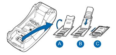
Figure 16 Inserting SIM Card
