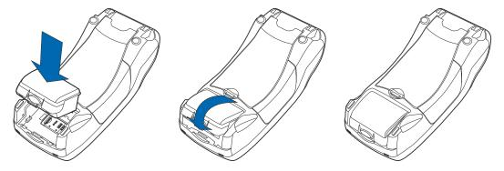
Figure 6 Installing the Smart Battery
