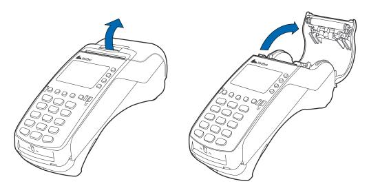
Figure 9 Opening the Printer Cover
