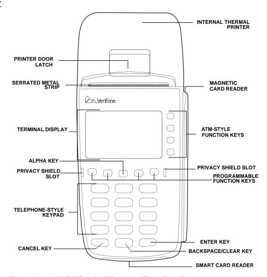
Figure 2 VX 520Terminal Features (Front Panel)
