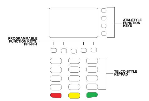
Figure 23 Front Panel Key Arrangement
