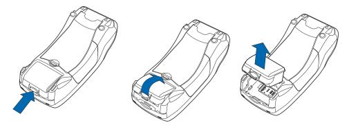
Figure 15 Removing the Smart Battery
