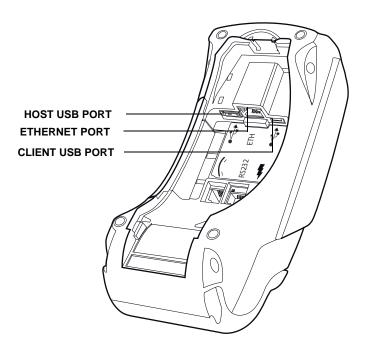
Figure 5 Additional VX 520 Connection Ports
