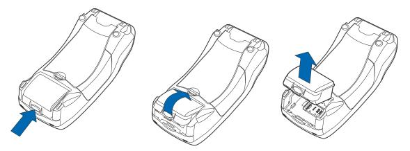
Figure 7 Removing the Smart Battery
