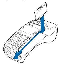
Figure 22 Using the Magnetic Card Reader
