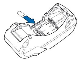
Figure 14 Installing an MSAM Card
