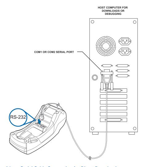
Figure 34 Serial Cable Connection for Direct Downloads
