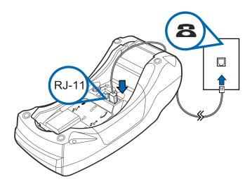
Figure 8 VX 520 Direct Telephone Connection
