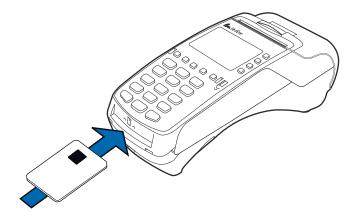
Figure 21 Inserting a Smart Card
