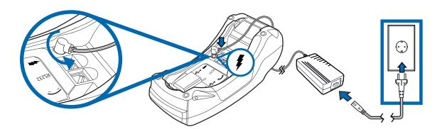
Figure 19 VX 520Power Pack Connection
